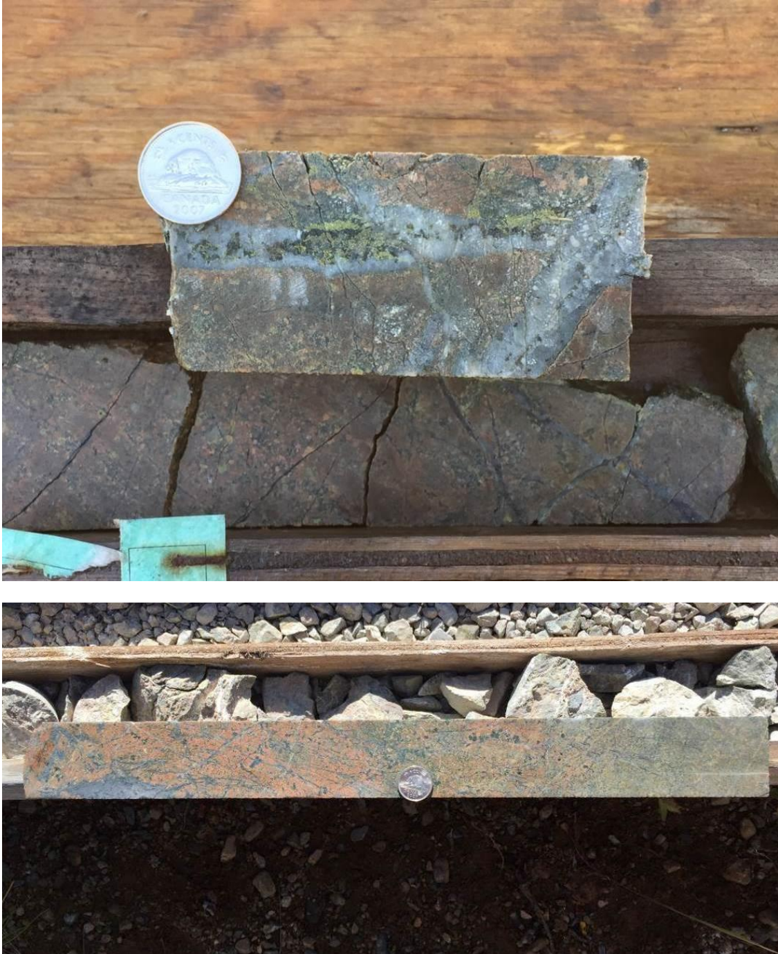
Figure 7-8: Quartz-magnetite-pyrite-epidote veinlets in potassic-altered latite (top: hole BR-03-07@165.95m) and quartz-magnetite±pyrite stockwork in hematite-dusted, weakly potassic-altered (right) to phyllic-altered (right) latite (bottom; hole BR-07-04@226.00m)
