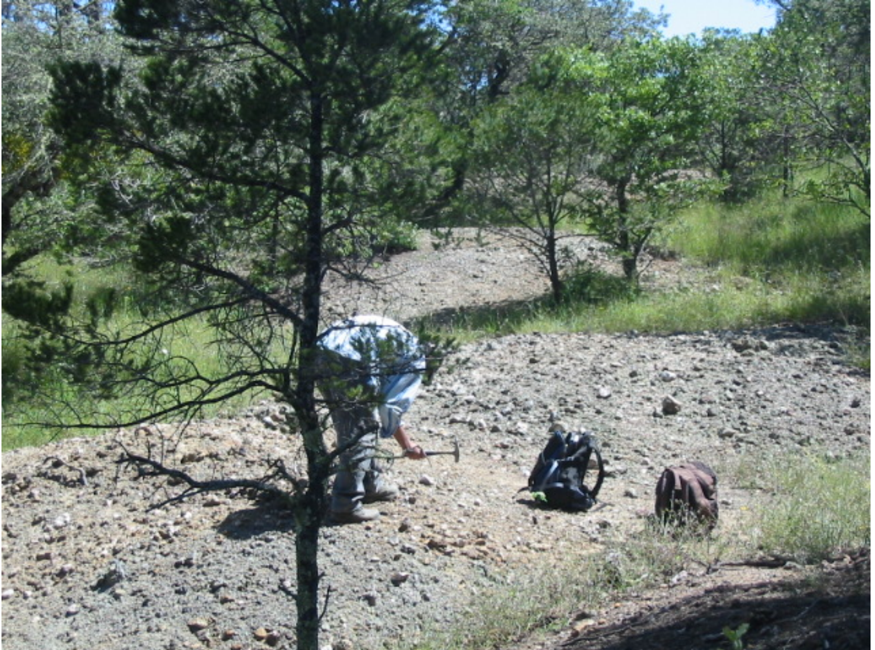
Mineral dump above the Barite vein Sample 485, 0.142 g/t Au, 253 g/t Ag, 2.36% Pb, 0.13% Zn
