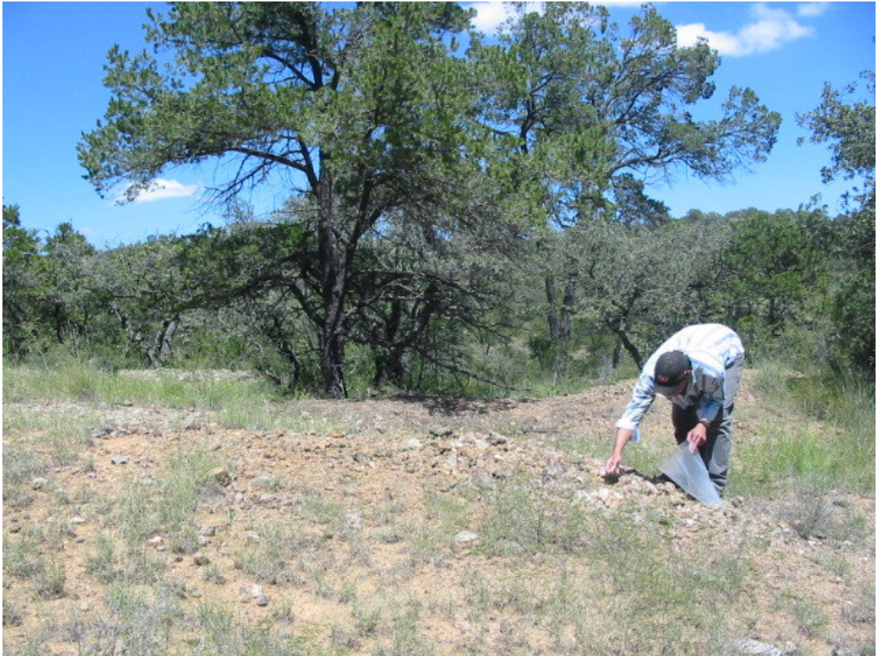
Mineral dumps above the Barite vein Sample 484, 0.06 g/t Au, 480 g/t Ag, 2.43% Pb, 0.3%Zn
