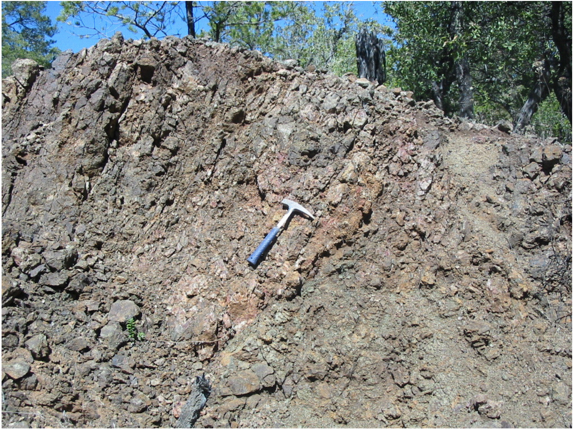
Maria Fernanda vein outcrop with width of about 1.5 meters; vuggy quartz with galena, chalcopyrite, malachite and iron oxides. Sample 447, 2.82 g/t Au-139g/t Ag-0.5%Cu
